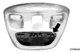
Use this button to select a readout of the outside temperature and one of eight compass headings that indicate the direction in which the vehicle is facing.
